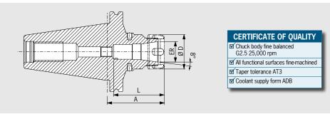
The Power Collet Chuck is designed for the highest machining capacity in High Speed manufacturing. The optimized design with improved construction combines high rigidity with vibration dampening features, giving more protection to the machine, spindle and tool. The universal Power Collet Chuck is a unique high performance chuck that can also be used with standard collets.
