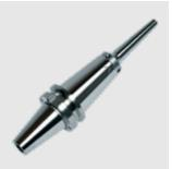
Power Mini Shrink Chuck is perfect for 5-axis machining in the die & mold and in the medical industry. Very slim at the top like the HAIMER Mini Shrink Chucks, the Power Mini Shrink is reinforced at the base. This allows for efficient milling with an angled tool, even at long protruding lengths.
