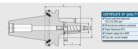
The Power Shrink Chuck is designed for the highest cutting performance in High Speed manufacturing. The optimized design combines high rigidity with vibration dampening, which protects the machine, spindle and tool.
