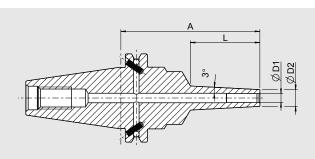
Power Mini Shrink Chuck is perfect for 5-axis machining in the die & mold and medical industry. Very slim at the top like the HAIMER Mini Shrink Chucks, the Power Mini Shrink is reinforced at the base. This allows for efficient milling with an angled tool, even at long protruding lengths.
