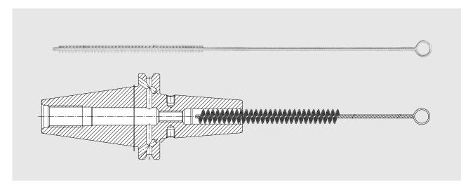
In order to achieve the best possible shrink fit connection, a grease free socket and shank is necessary. The cleaning can be done by a cold solvent (e.g. brake cleaner). An appropriate cleaning brush is necessary to clean the socket of the Shrink Fit Chuck.
