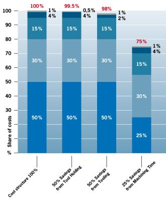
The result: The costs for tooling and tool holders are nearly meaningless. Even with savings of 50%, the total costs remain nearly the same.
