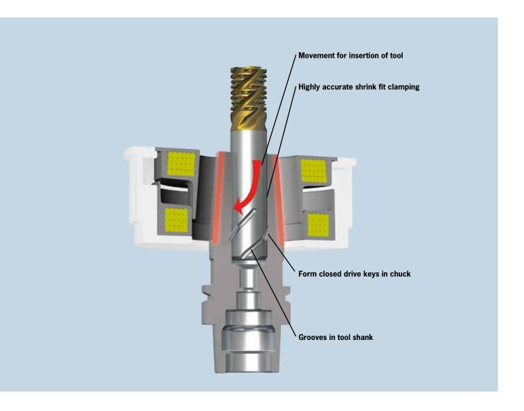
The following tool manufacturers are licensed by HAIMER officially and offer their shank cutting tools with Safe-Lock grooves in the tool shank as a standard.
