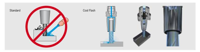
True to the slogan "make good things even better", HAIMER has developed the Cool Flash system out of the existing Cool Jet system. The Cool Flash design directs coolant into T-slots at the nose of the holder and works with the centrifugal force of the rotating tool to lead the coolant along the shank of the cutter and directly to the flutes at any speed.
