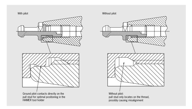
HAIMER goes far beyond the requirements of CAT40 tooling. Our experience with tool holders and balancing have merged together to successfully create far superior CAT tapered tooling.
