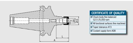
The High Precision Collet Chuck is the collet chuck for highest metal removal rates in High Speed cutting. The optimized design with better construction and a special coated smooth locknut combines high rigidity with vibration dampening and noise-reducing features, giving more protection to machines, spindles and tools.
