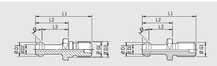
Version with ground pilot is used to help consistently locate the pull stud in the tool holder. Great for runout accuracy, balance repeatability and machine tool draw bar consistency.
