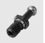
Version with ground pilot is used to help consistently locate the pull stud in the tool holder. Great for runout accuracy, balance repeatability and machine tool draw bar consistency.
