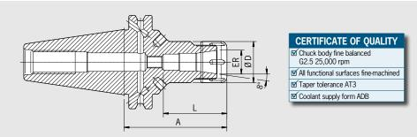
The Power Collet Chuck is designed for the highest machining capacity in High Speed manufacturing. The optimized design with improved construction combines high rigidity with vibration dampening features, giving more protection to the machine, spindle and tool. The universal Power Collet Chuck is a unique high performance chuck that can also be used with standard collets.
