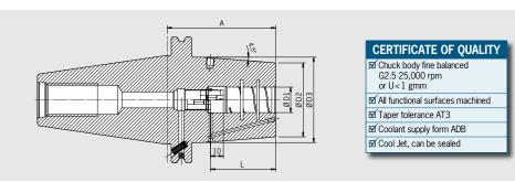
Finally there is a holder for heavy machining that can replace the Weldon tool holder. The Heavy Duty Chuck is a shrink fit chuck designed for extreme cases. The contour is optimized for highest rigidity and clamping force.
