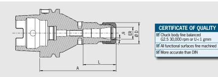
The High Precision Collet Chuck is the collet chuck for highest metal removal rates in High Speed cutting. The optimized design with better construction and a special coated smooth locknut combines high rigidity with vibration dampening and noise-reducing features, giving more protection to machines, spindles and tools.
